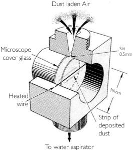
Figure 17: (above) A thermal precipitator used for sampling the concentration of airborne dust, designed by the National Coal Board, being checked by members of the PRU, 1940s, (below) Sampling head.
