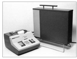
Figure 53: Litton Monroe Epic 3000 keyboard and printing unit with free-standing calculating unit, introduced in 1967 as the first programmable printing calculator. © Nigel Tout.
